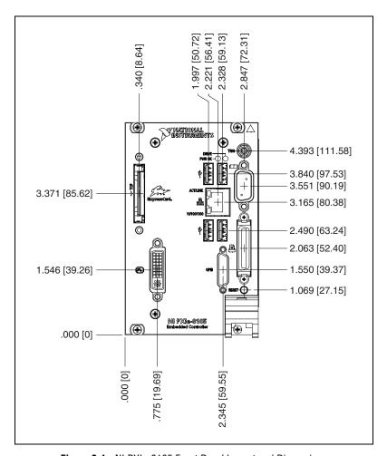
Figure 3-1. NI PXIe-8105 Front Panel Layout and Dimensions
